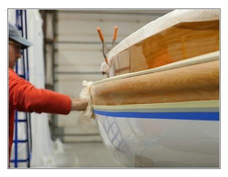
Before applying varnish, do one last solvent wipe to remove contaminants, and allow the surface to dry completely. Wipe the surface with a clean, lint-free rag dampened with <u>TotalBoat Special Brushing</u> <u>Thinner 100</u>.
