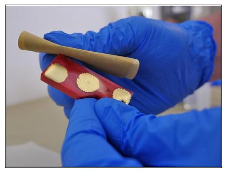
If you have a couple of edges that need to be a little smoother, sand lightly with <u>320-grit sandpaper</u>. Be sure to wear a dust mask or N95 respirator when sanding cured epoxy.
