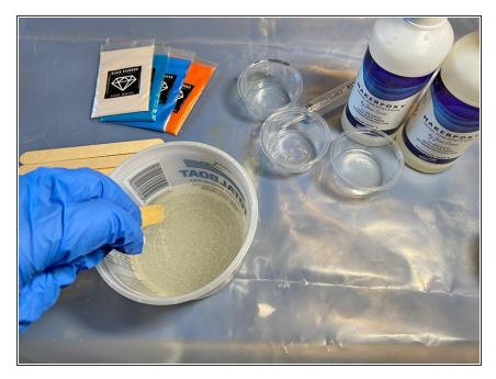
Dispense 1 part TotalBoat MakerPoxy Epoxy Resin to 1 part TotalBoat MakerPoxy Epoxy Hardener (by volume) into a clean mixing cup.
