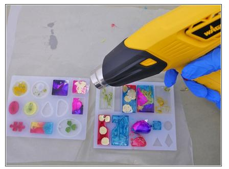
To pop any small air bubbles, wave <u>the heat gun</u> (on low setting) quickly, back and forth above the surface, and keep it moving. This only takes a couple of seconds.
