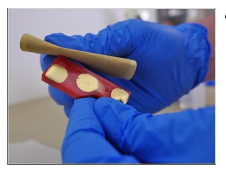
If you have a couple of edges that need to be a little smoother, sand lightly with <u>320-grit sandpaper</u>. Be sure to wear a dust mask or N95 respirator when sanding cured epoxy.
