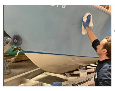
it's important to remove all previous wax and contamination from the boat before you apply rubbing compound. Different finishes will require different products, as described below.
