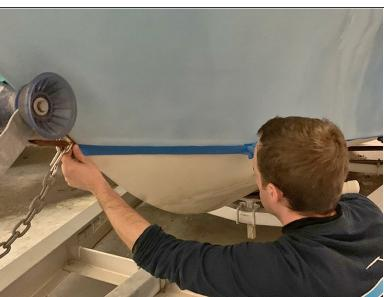
To prevent bottom paint from getting rubbed around in the polish and wax, mask below the waterline. Be sure to use a <u>quick-release masking tape</u> that won't leave residue.
