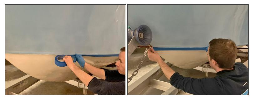
To prevent bottom paint from getting rubbed around in the polish and wax, mask below the waterline. Be sure to use a <u>quick-release masking tape</u> that won't leave residue.
