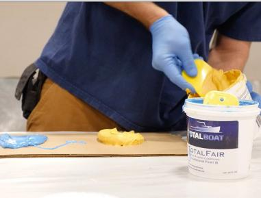
Always start with clean tools and mixing surfaces. Combine the <u>TotalFair</u> yellow epoxy resin (Part A) and blue hardener (Part B) at the specified mix ratio of 1 to 1 by volume (1 part resin to 1 part hardener). There is a small tolerance if the mix is not exactly 1:1 – just do the best you can to make sure the amounts look equal.
